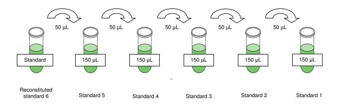
After serial dilutions, the tubes should have the following concentrations for constructing standard curves.
