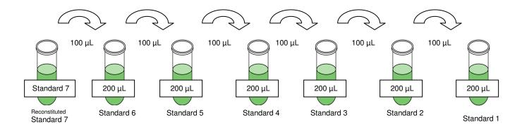
After serial dilution, the tubes should have the following concentrations for constructing standard curves.
