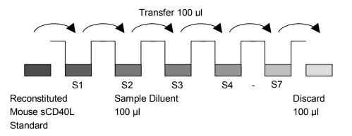
In case of an <u>external standard dilution</u> (see 9.5.1), pipette 100  $\mu$ l of these standard dilutions (S1 - S7) in the standard wells according to Table 1.
