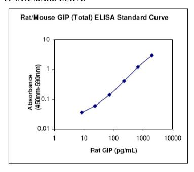
Typical Standard Curve, not to be used to calculate results.
