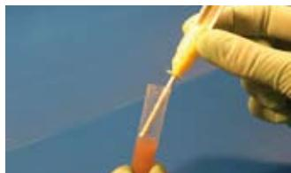
Turn the cone containing the dosing tip counter-clockwise and remove by pulling it upwards.
