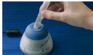
Homogenize the sample by vortexing for 30 sec., let it stand for 10 min. and vortex again for 30 sec. using a vibration mixer. Repeat this step until the faeces has completely been removed from the dosing tip.
